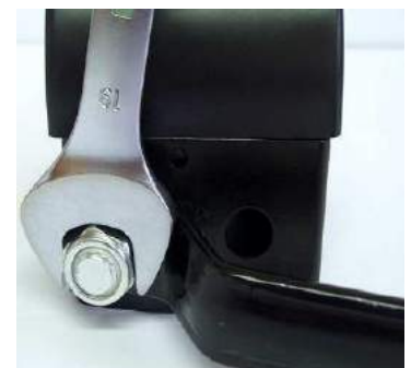
Figure 9 – Crank handle setting Montage manivelle
