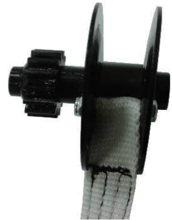
Figure 7 – Assembly drum+strap Ensemble bobine-sangle
