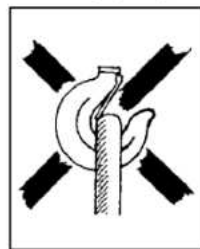
Fig 2 c Hook latch obstructed
